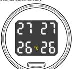
The display will show temperature unit °( if the tire temperature is above  $0^{\circ}$ C, and will show  ${}^{\circ}$ C if it is under  $0^{\circ}$ C.
